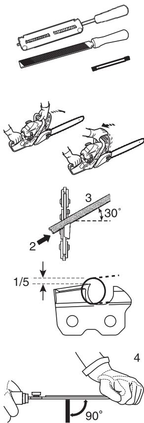
1. Lock the chain - push the front hand guard forward.
