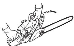
1. Place the chain saw on the ground.
